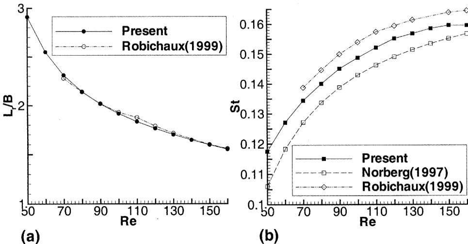
Figure 10. Variation of (a) mean recirculation length and (b) Strouhal number with Reynolds number for the periodic flow.
