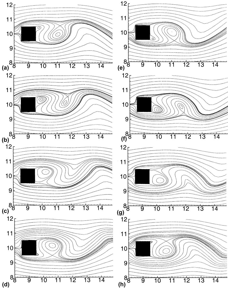
**Figure 5.** Instantaneous streamlines near the square cylinder, separated by an interval of one-eighth of the time period of vortex shedding, at  $Re = 100$ .
