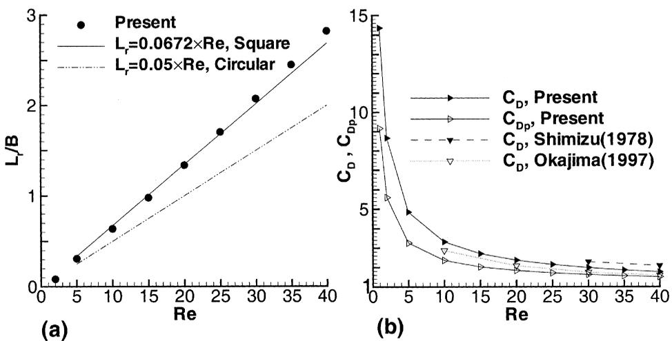
**Figure 9.** Variation of (a) recirculation length and (b) coefficient of total and pressure drag with Reynolds number for the steady flow.
