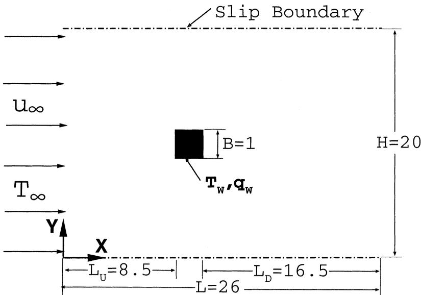
Figure 1. Computational domain for the flow around a square cylinder and the associated parameters.
