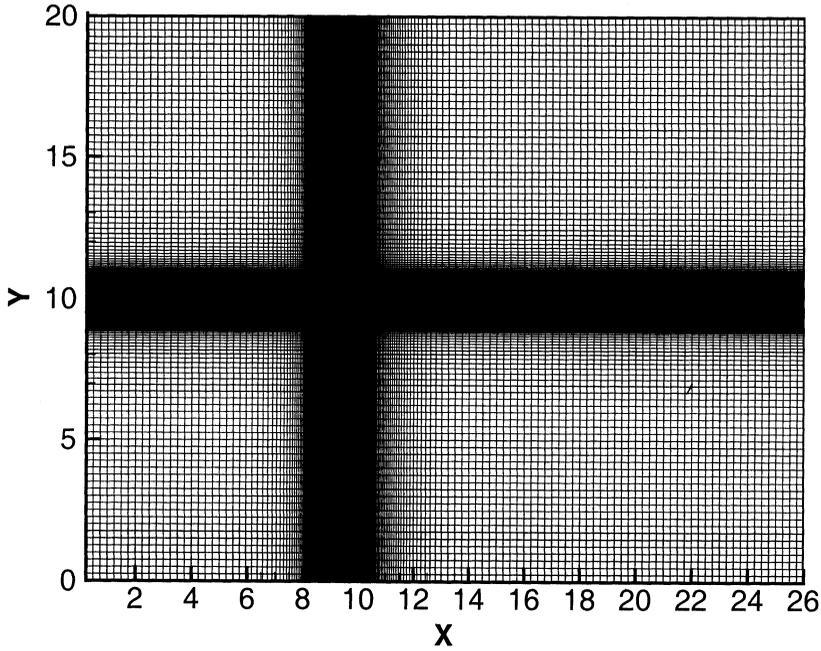
Figure 2. Non-uniform computational grid structure with  $323 \times 264$  grids.
