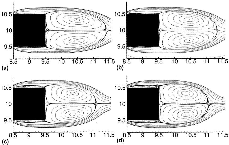
**Figure 6.** Time-averaged streamlines near the square cylinder at (a)  $Re = 100$ ; (b)  $Re = 110$ ; (c)  $Re = 150$ , and (d)  $Re = 160$  (inviscid saddle points, near the rear end corner, are marked by a circle).
