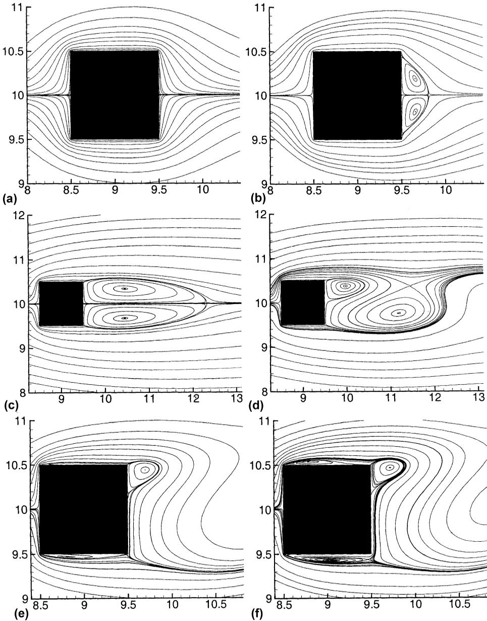
**Figure 4.** Streamlines (instantaneous for the periodic flow) around the square cylinder for different Reynolds numbers: (a)  $Re = 1$ ; (b)  $Re = 2$ ; (c)  $Re = 40$ ; (d)  $Re = 50$ ; (e)  $Re = 120$ ; (f)  $Re = 160$ .
