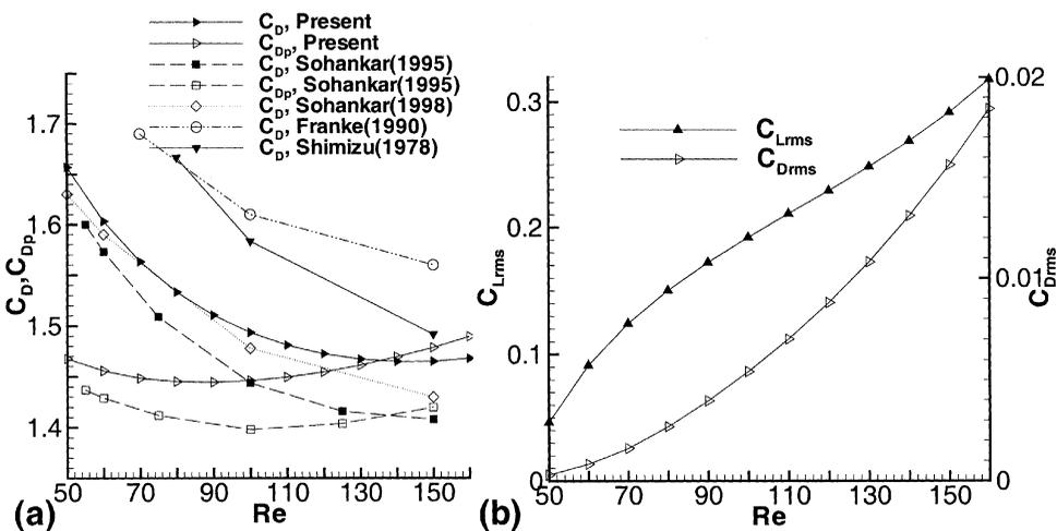
**Figure 11.** Variation of (a) time-averaged value of coefficient of total drag and pressure drag and (b) rms value of lift and drag coefficient with Reynolds number for the unsteady periodic flow.
