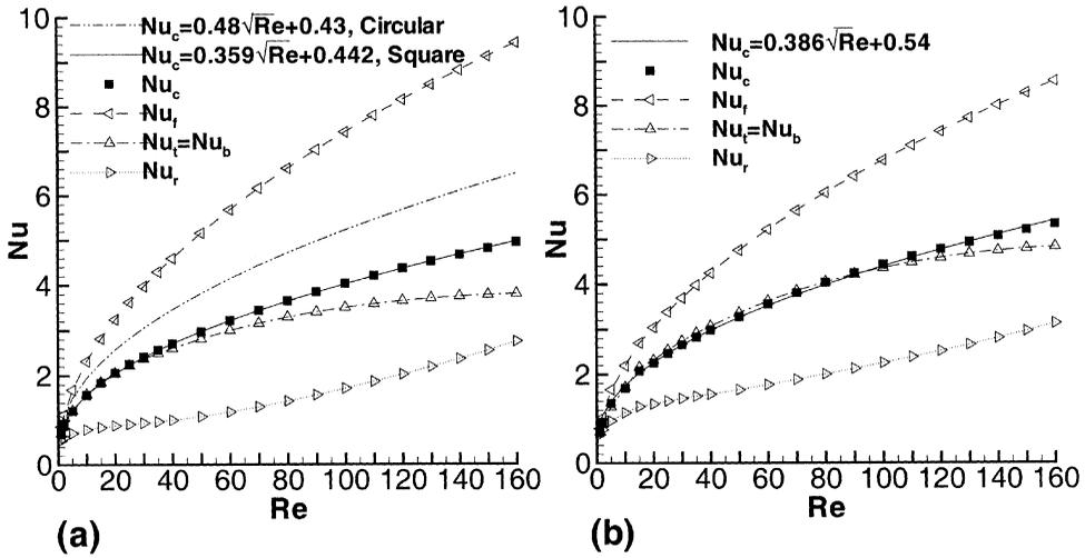
**Figure 12.** Nusselt number (time-averaged for the periodic flow) for the cylinder and each of its face as a function of Reynolds number for (a) constant cylinder temperature case and (b) constant heat flux case. Subscripts: f, front; t, top; r, rear; b, bottom; c, cylinder average.
