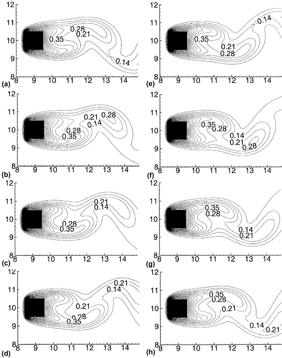
**Figure 7.** Instantaneous isotherms near the square cylinder, separated by an interval of one-eighth of the time period of vortex shedding, at  $Re = 100$ , for the constant cylinder temperature case.
