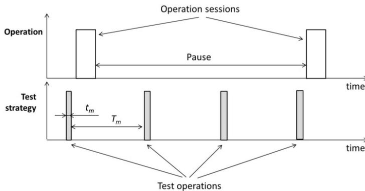
Fig. 3. Time diagram of sensor node operation and its testing.
