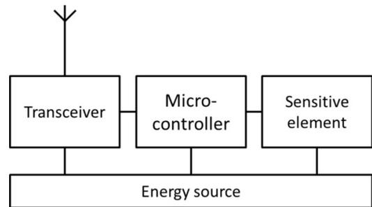
Fig. 2. Sensor node inner structure<sup>2</sup>.
